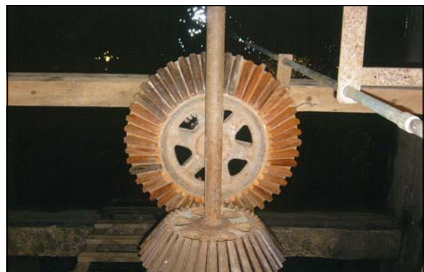
Below: The new wooden turbine teeth are helping to run the wheel at Wagaman Mill. The wooden teeth run with the metal gear to operate the pulleys and belts inside the wheelhouse.
