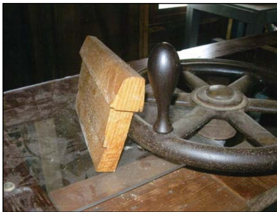
Above: A new turbine tooth made of oak by Walt Van Maanen.
